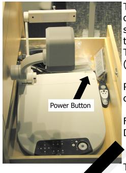
The document camera is located on the side of the lectern. Unlock the side panel, and slide out the document camera drawer. Lift the light and head of the document camera. The camera can display any type of object (photos, coins, papers, etc).
