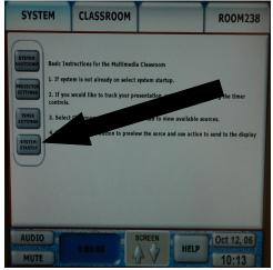
Tap the "System Startup" button. The system will power up, the screen will lower, and the projector will power up. Projector settings are set automatically, there's no need to adjust them.
