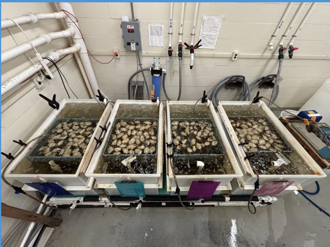
Figure 3 - Heat shock experiment tank set-up for adult clams.
