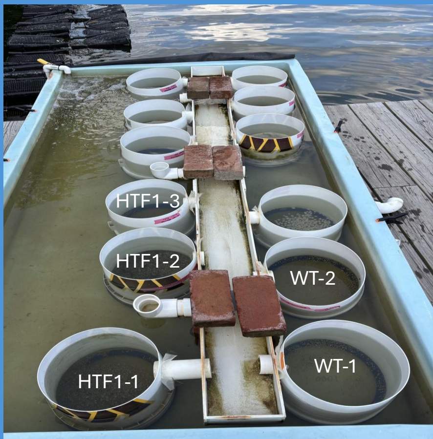
Figure 4 - Heat shock experiment tank set-up for juvenile clams.
