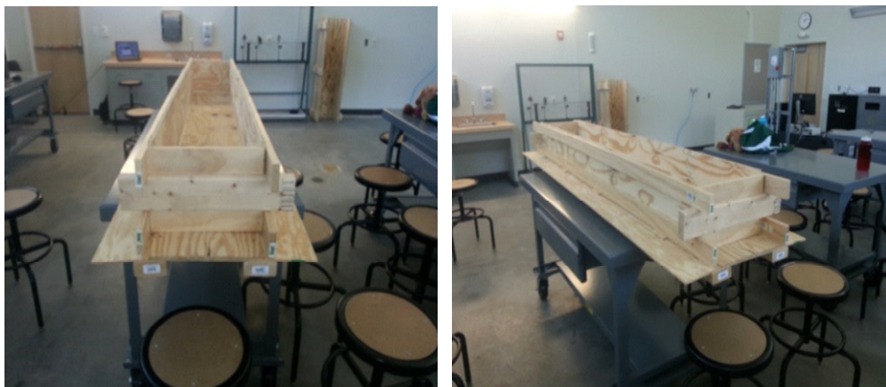
Fig. 1: Formwork for 7' beams to be prestressed with AFRP bars
