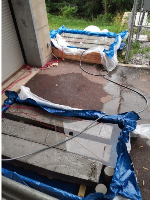
Fig. 9: Beams in the wet phase of the wet/dry cycle
