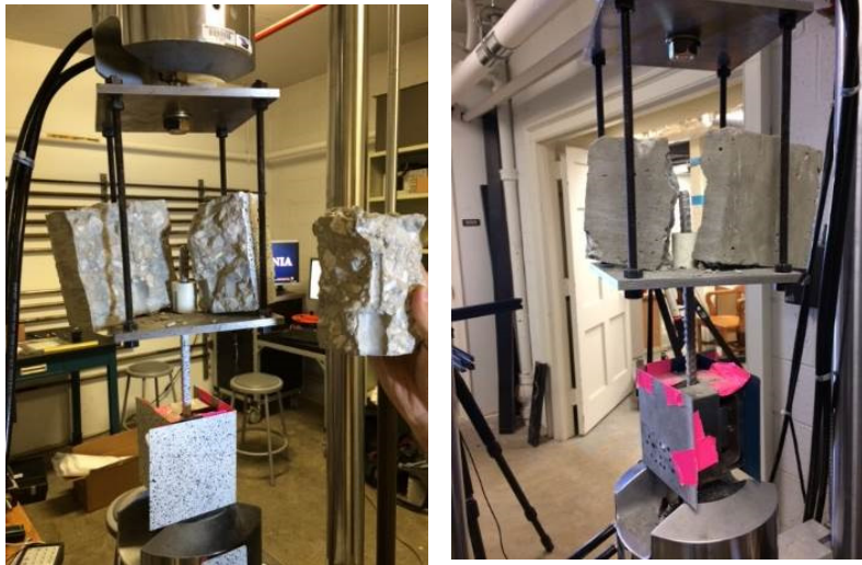
Fig. 13: Concrete failures during testing due to concrete quality and embedded rebar alignment
