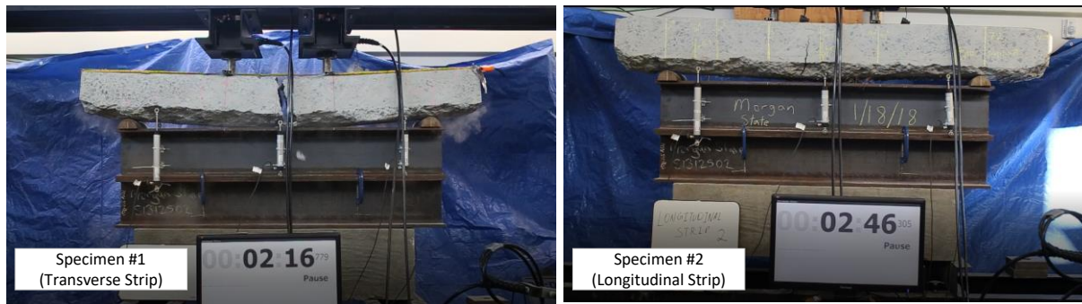
Figure 23. Tests results of transverse and longitudinal specimens, (a) load-time response and comparison between theoretical calculation and test, (b) specimen #1/ transverse strip at break point, (c) specimen #2/ longitudinal strip at break point
