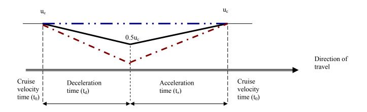
• = Deceleration-acceleration profile of vehicles arriving at the end of bus stopping maneuver
