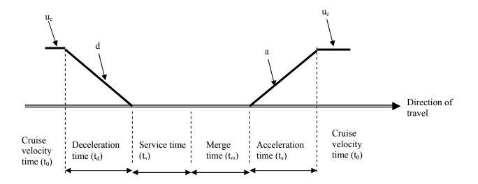
Figure 2 Schematic illustration of bus velocity profile at bus stops
