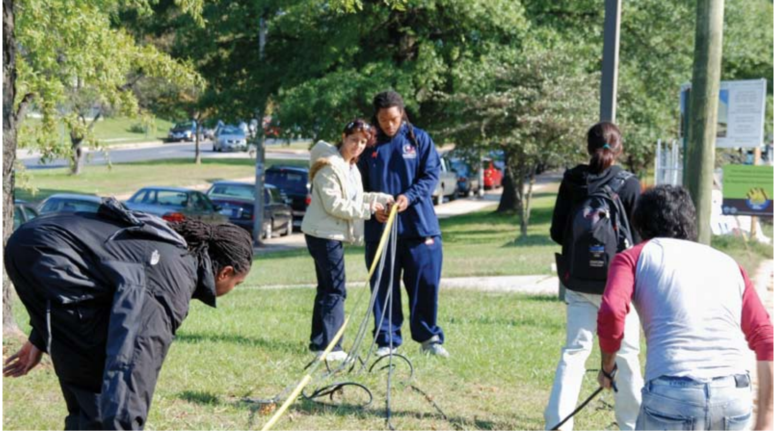
Dr. Mansoureh Jeihani's project Evaluating the Effectiveness of Dynamic Speed Display Signs investigates whether the signs slow drivers. In October 2010, Dr. Jeihani and her research assistants installed tubes and counting devices on Perring Parkway (between Echodale Avenue and Northern Parkway) to track the speed of cars approaching and passing the devices. Photo by Dean Eugene DeLoatch.
